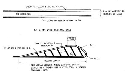
DIAGONAL LINE SPACING: 15 m (50') C-C (LESS THAN 50 km/h (30 MPH)) 25 m (75') C-C (50 km/h (30 MPH) TO 70 km/h (45 MPH)) 45 m (150') C-C (MORE THAN 70 km/h (45 MPH))
