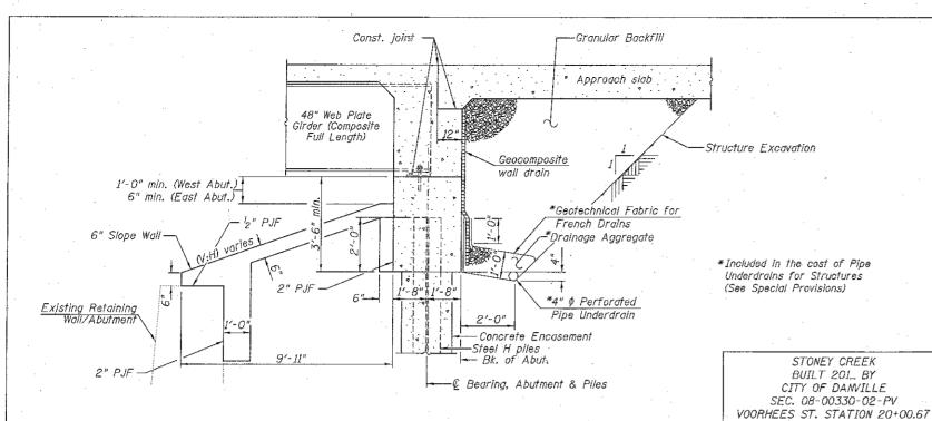
All drainage system components shall extend to inside face of each existing wingwall except the \*pipe underdrain shall extend to the outside face of existing wingwalls. A \*hole shall be drilled into the existing wingwalls for the pipe underdrain to exit through.
