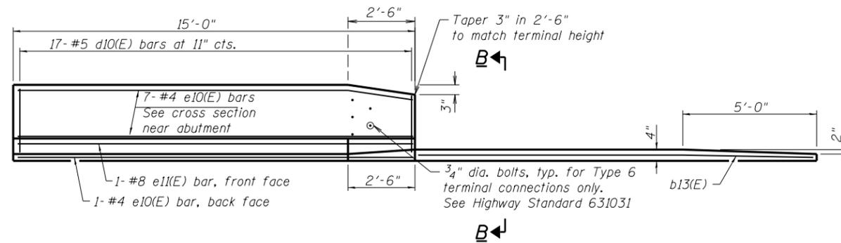
**INSIDE ELEVATION OF PARAPET AND CURB**
