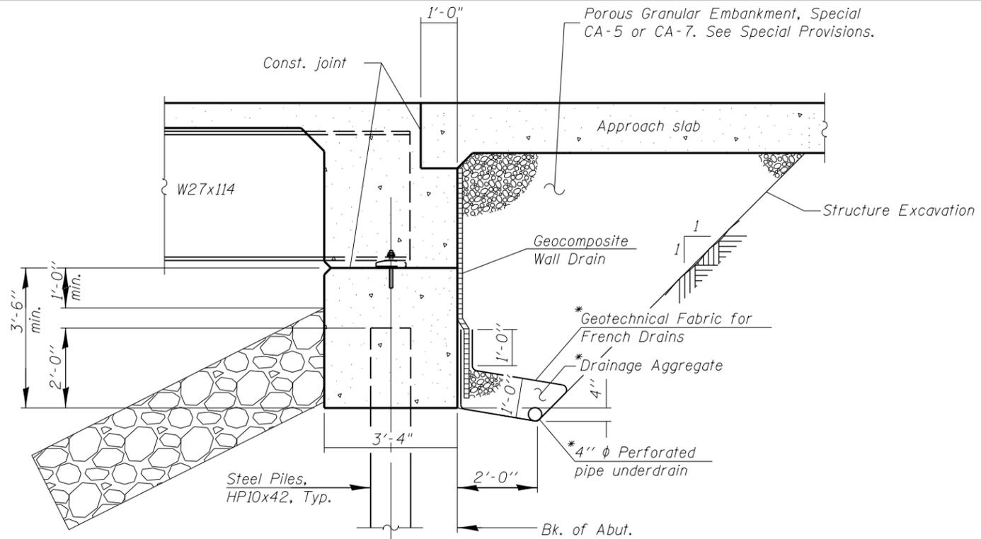
**SECTION THRU INTEGRAL ABUTMENT**
