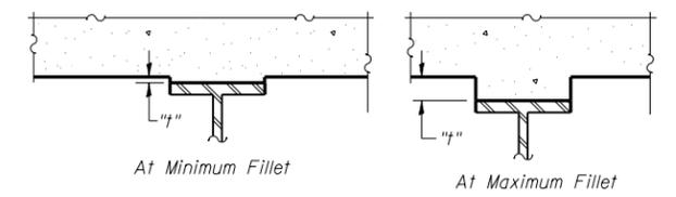
To determine "f": After all structural steel has been erected, elevations of the top flanges of the beams shall be taken at intervals shown on sheets 22 & 23 of 29. These elevations subtracted from the "Theoretical Grade Elevations Adjusted for Dead Load Deflection" shown below, minus slab Thickness, equals the fillet heights "f" above top Flange of Beams.
