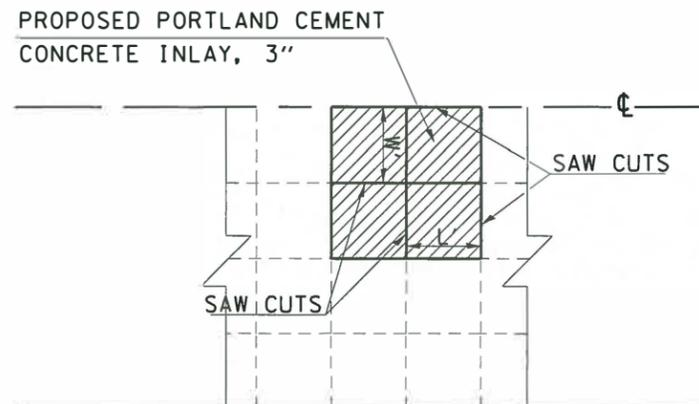
SAW CUTS SHALL BE MADE AT ALL EXISTING JOINTS FOR PAVEMENT REMOVAL (SPECIAL) AND FOR PORTLAND CEMENT CONCRETE INLAY, 3"
