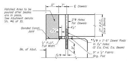
\* Dowel Rods to be grouted after beams are in place and allowed to cure (Min. 24 hr.) prior to grouting the shear keys.
