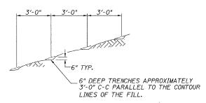
NOTE: ALL SLOPES 3:1 OR STEEPER AND GREATER THAN 5' IN HEIGHT SHALL BE CONTOUR PLOWED AS SHOWN IN DETAIL, COST SHALL BE INCLUDED WITH SEEDING, CLASS 2 (SPECIAL).
