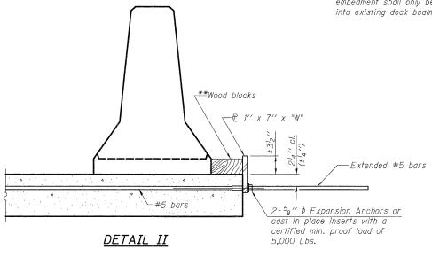
\*\* Wood blocks may be omitted when required to provide minimum stage traffic lane width. When the wood blocks are omitted, the concrete barrier shall be in direct contact with the steel retainer plate.
