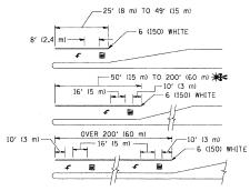
JURN LANES IN EXCESS OF 400' (120 m) IN LENGTH MAY HAVE AN ADDITIONAL SET OF ARROW - "ONLY" INSTALLED MIDWAY BETWEEN THE OTHER TWO SETS OF ARROW - "ONLY".
