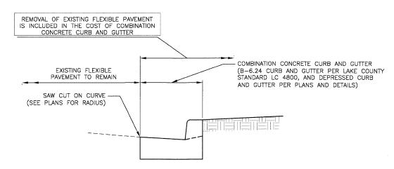
CURB AND GUTTER TYPICAL SECTION DETAIL B
