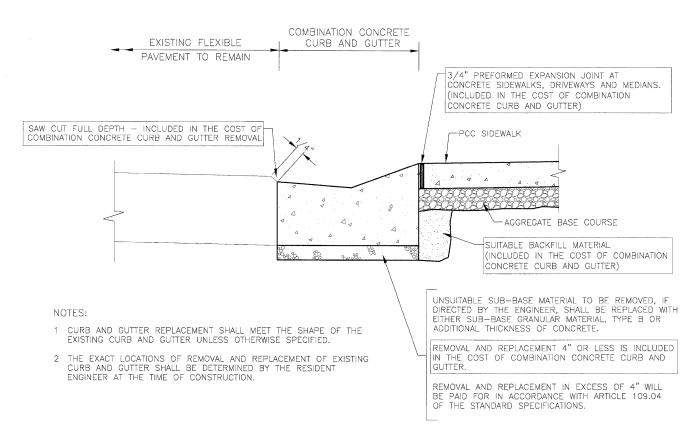
COMBINATION CONCRETE CURB AND GUTTER REMOVAL, AND COMBINATION CONCRETE CURB AND GUTTER
