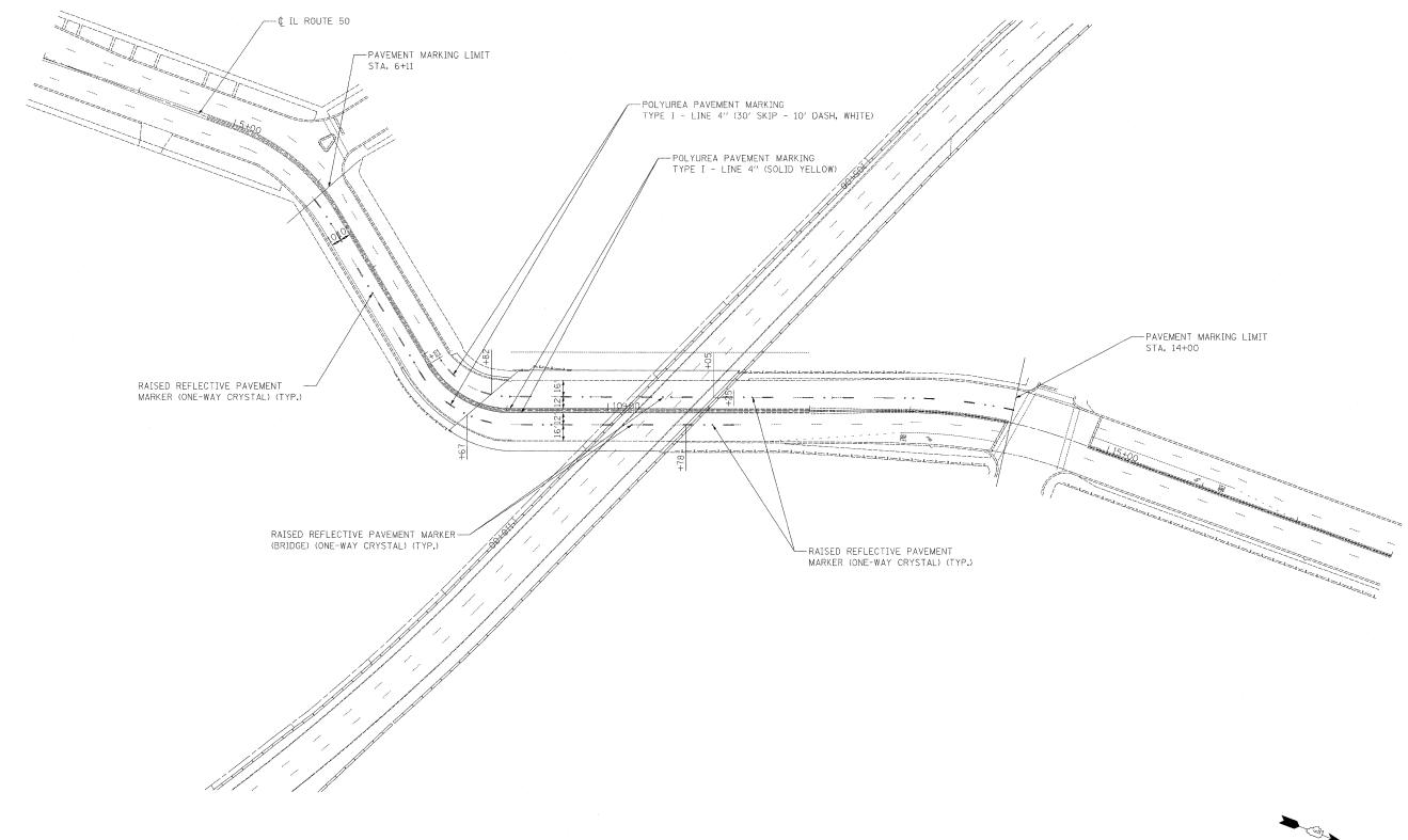
PROPOSED PAVEMENT MARKINGS AND RAISED REFLECTIVE PAVEMENT MARKERS ARE TO BE INSTALLED IN ACCORDANCE WITH HIGHWAY STANDARD 780001-03 AND DISTRICT ONE STANDARDS TC-11 AND TC-24.
