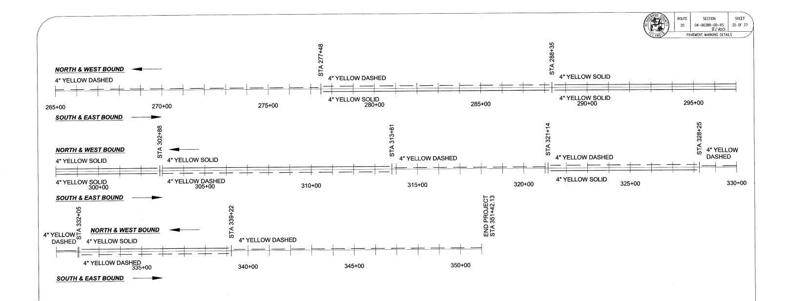
NOTE: STATIONING TO BE FIELD VERIFIED BY THE ENGINEER PRIOR TO PLACING THE STRIPING AND SHALL BE IN ACCORDANCE WITH THE MUTCD.
