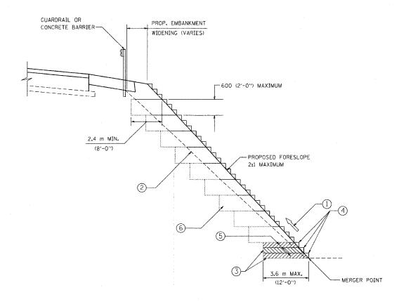
TYPICAL BENCHING DETAIL FOR EMBANKMENT
