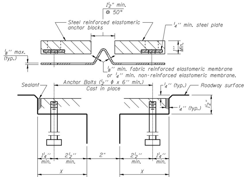
**CROSS SECTION DETAIL A EXISTING JOINT**
