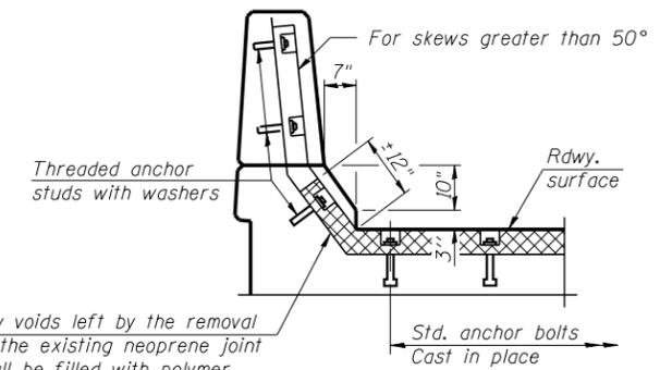
Any voids left by the removal of the existing neoprene joint shall be filled with polymer concrete.
