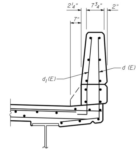
**EXISTING SECTION THRU PARAPET**
