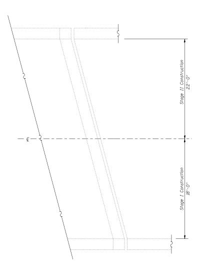
PROPOSED PARTIAL PLAN Joint at South Abutment
