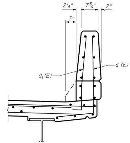
**EXISTING SECTION THRU PARAPET**
