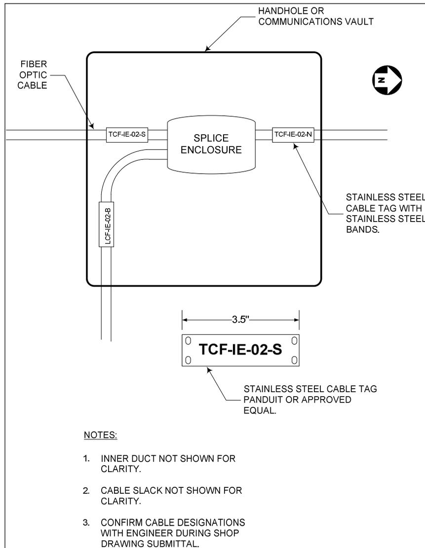
Label the destination of each trunk cable onto the cable in each handhole, vault or cable termination panel.
