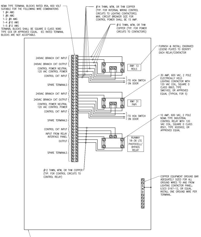
NEMA 4X STAINLESS STEEL OR ALUMINUM ENCLOSURE WITH HINGED DOOR SIZED AS REQUIRED TO HOUSE LIGHTING CONTACTORS, CONTROL RELAY, TERMINAL BLOCKS, WIRING & INTERFACE TO EXISTING CONDUITS, APPROXIMATE 24"Hx20"Wx8"D AS MANUFACTURED BY HOFFMAN OR APPROVED EQUAL CONFIRM DIMENSIONS AND PROVIDE AN ENCLOSURE TO HOUSE EQUIPMENT AND TO FIT INSIDE VAULT TRANSCLOSURE. NOTE - NEMA 4X RATING IS TO ACCOMMODATE FUTURE RELOCATION TO AN OUTDOOR
