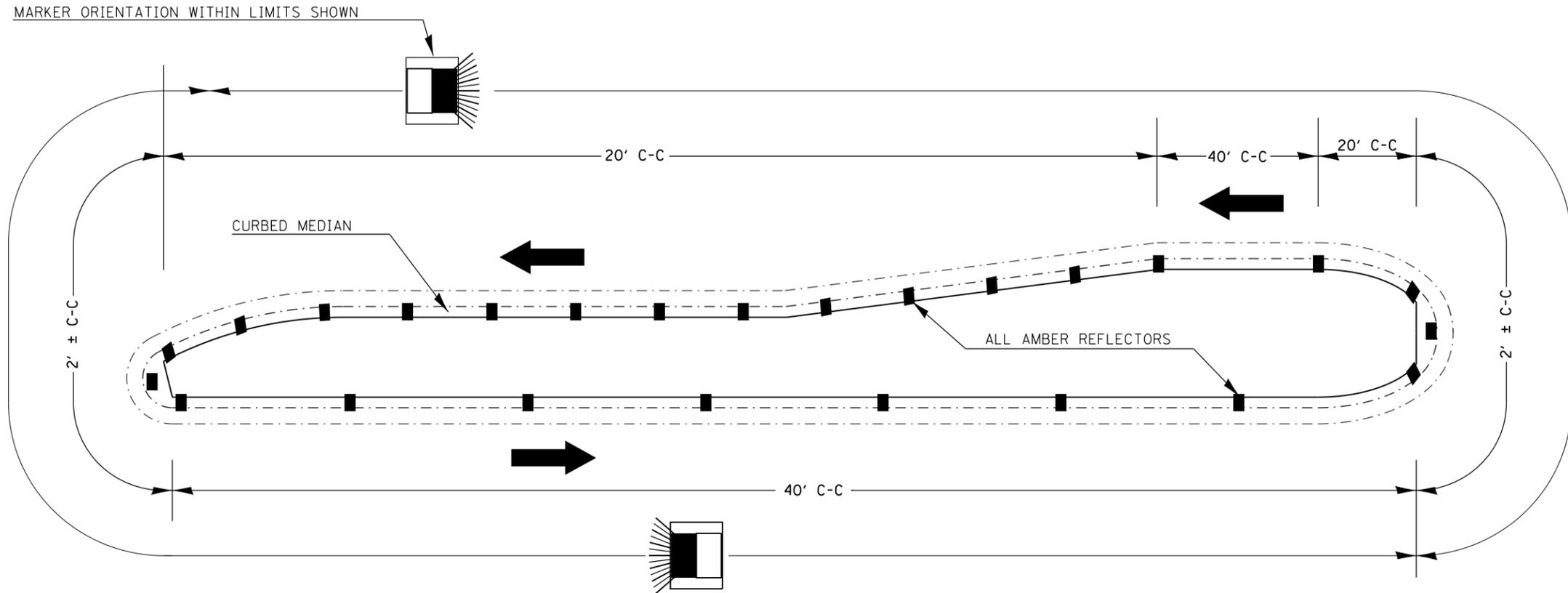
1. PRISMATIC REFLECTORS SHALL BE MONO-DIRECTIONAL AND POSITIONED SO THAT THE REFLECTIVE FACE IS FACING THE APPROACHING TRAFFIC.
