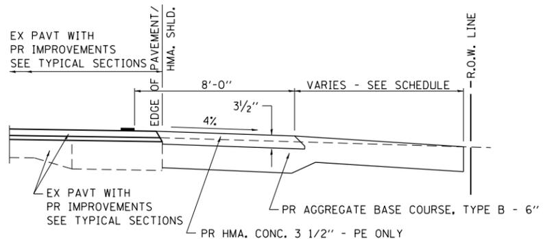
**SECTION A-A FOR EX EARTH/AGGREGATE FE & PE**
