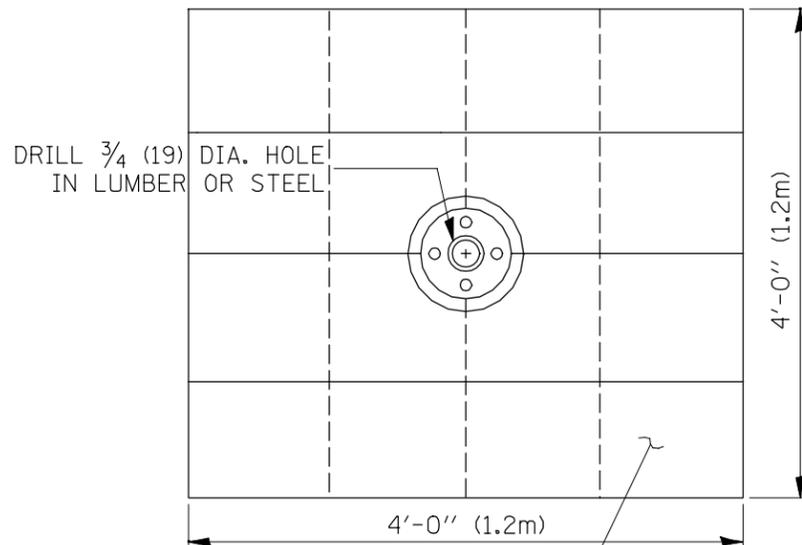
SOUND LUMBER - 1(25) x 12(300) NAILED TOGETHER OR 1/4(6) THICK BY 4'(1.2m) SQUARE STEEL PLATE
