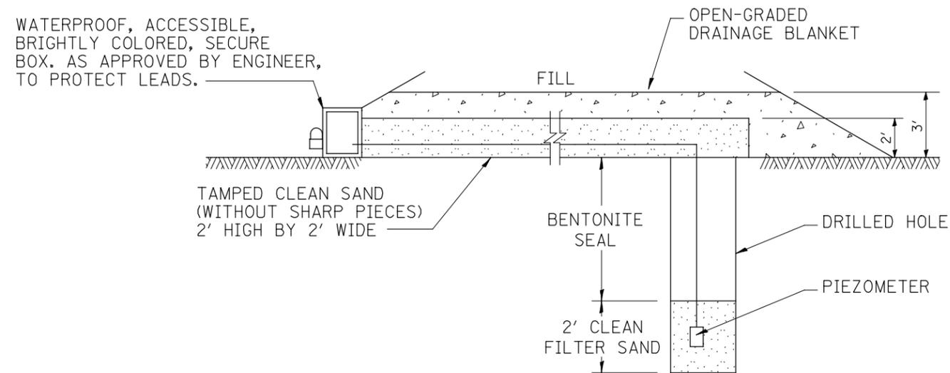
TYPICAL PIEZOMETER INSTALLATION DETAIL
