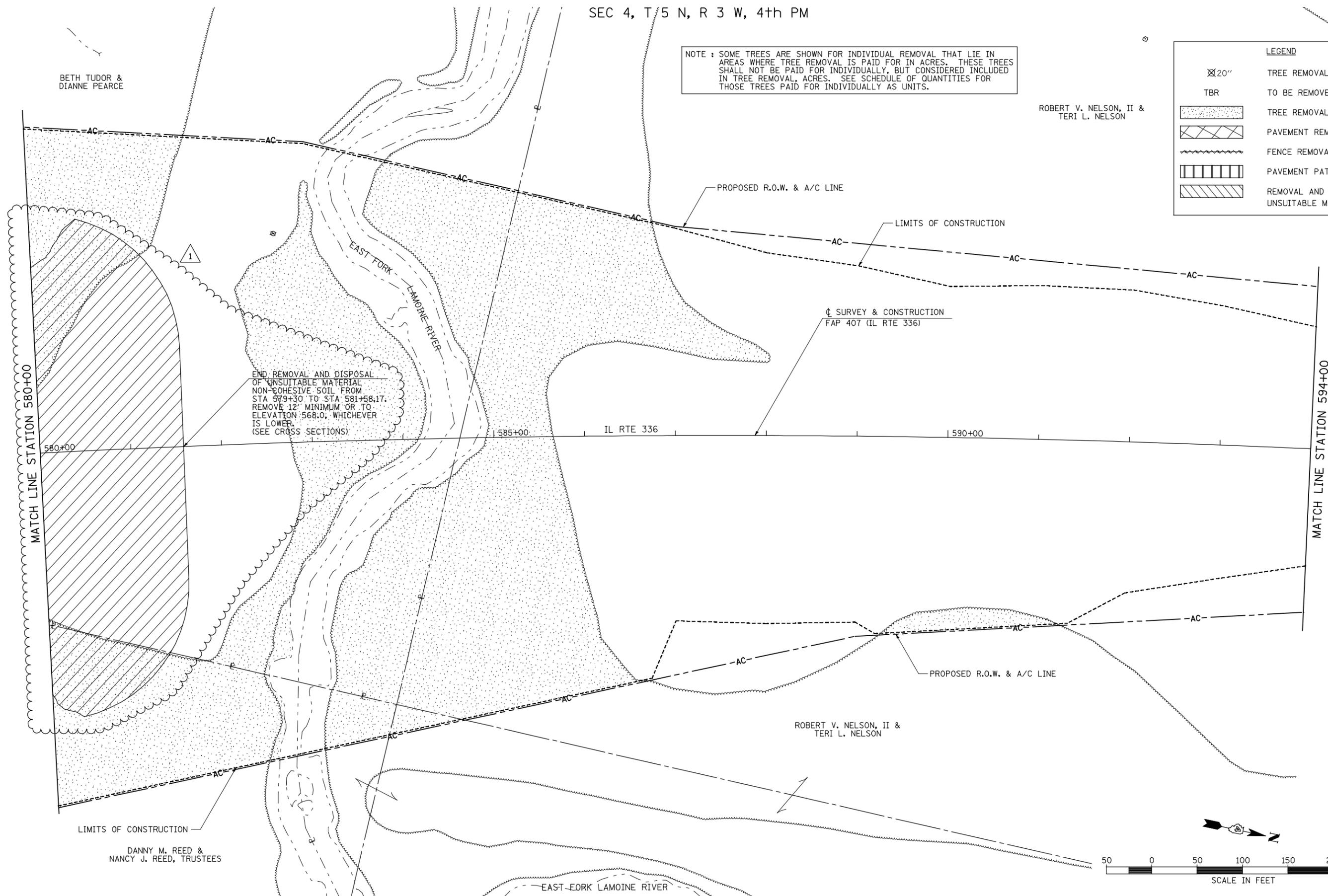
END REMOVAL AND DISPOSAL OF UNSUITABLE MATERIAL NON-COHESIVE SOIL FROM STA 579+30 TO STA 581+58.17. REMOVE 12" MINIMUM OR TO ELEVATION 568.0, WHICHEVER IS LOWER. (SEE CROSS SECTIONS)
