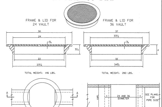
ALTERNATE MATERIALS FOR WALLS BRICK MASONRY CAST-IN-PLACE CONCRET CONCRETE MASONRY UNIT PRECAST REINFORCED CONCRETE SECTION
