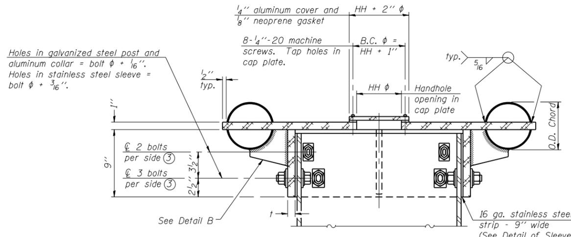
④ Collar I.D. shall be manufactured to correspond to O.D. of actual galvanized post and stainless steel sleeve plus 1/8" (±1/16"). Maximum gap between post and collar at any location equals 1/8" before tightening bolts.
