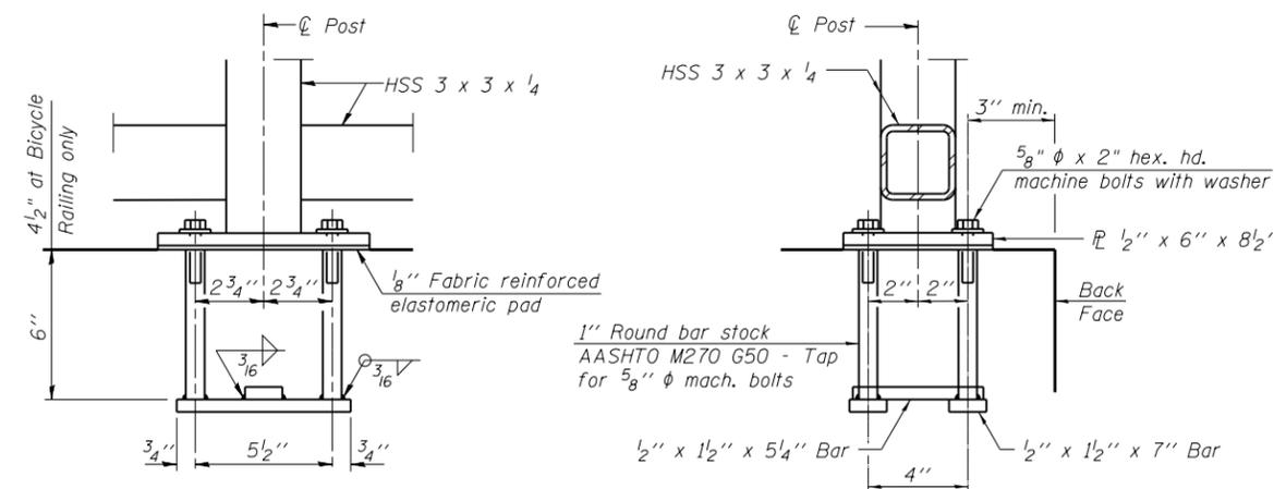
In lieu of the cast-in-place anchor device shown, the Contractor has the option of drilling and setting 5/8"  $\varnothing$  anchor rods according to Article 509.06 of the Standard Specifications. Embedment shall be according to the manufacturer's specifications, but no greater than 6".
