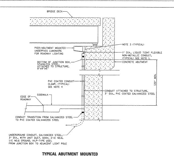
TYPICAL UNDERPASS LUMINAIRE AND JUNCTION BOX MOUNTING DETAIL NOT TO SCALE
