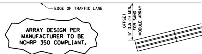
**ARRAY DESIGN PER MANUFACTURER TO BE NCHRP 350 COMPLIANT.**
