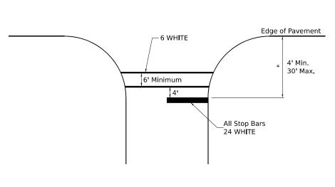
Distance to the nearest edge of the intersecting roadway in the absence of a marked crosswalk.
