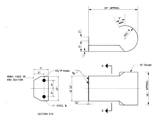
ALL OTHER STEEL SHAPES AND PLATES SHALL CONFORM TO THE REQUIREMENTS OF A.A.S.H.T.O. DESIGNATION M-183 EXCEPT POSTS AND ANGLES SHALL CONFORM TO A.A.S.H.T.O. M-223, GRADE 50.
