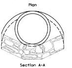
NOTE: FOR PLACEMENT, QUALITY GRADATION AND OTHER MISCELLANEOUS REQUIREMENTS FOR STONE RIPRAP DITCH-SEE SPECIAL PROVISIONS.
