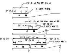
\* TURN LANES IN EXCESS OF 400' (120 m) IN LENGTH MAY HAVE AN ADDITIONAL SET OF ARROW - "ONLY" INSTALLED MIDWAY BETWEEN THE OTHER TWO SETS OF
