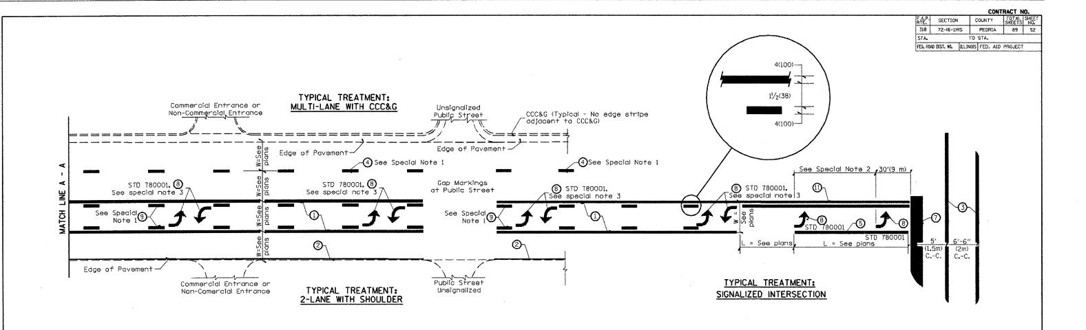
FLUSH PAVED MEDIAN: TWO-WAY LEFT TURN LANE WITH ONE-WAY LEFT TURN LANE AT SIGNALIZED INTERSECTION
