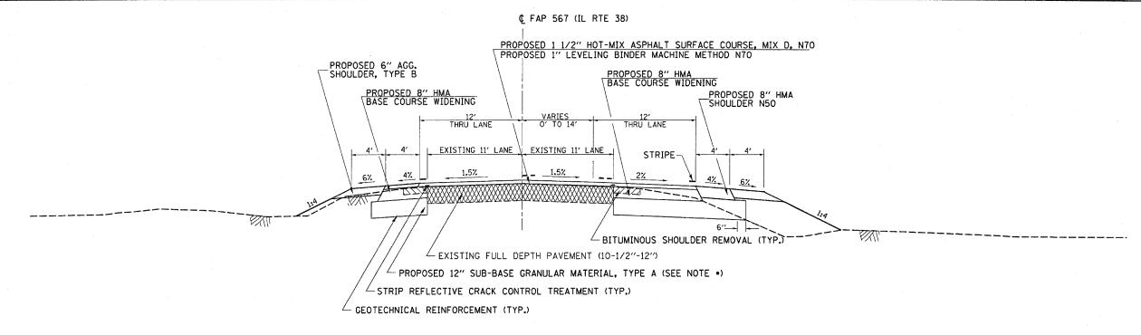
• STA 311+75 - STA 315+25 18" AGGREGATE SUB-BASE GRANULAR MATERERIAL, TYPE A
