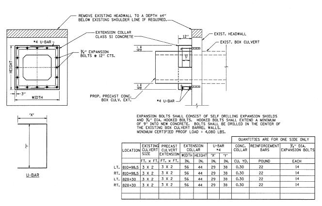
COLLAR DETAIL (PRECAST BOX CULVERT EXTENSION OF BOX CULVERT)
