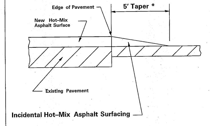
HOT-MIX ASPHALT APPLICATION RATES: All Hot-Mix Asphalt Mixtures: 112lb/sq. yd/inch Bituminous Materials (Prime Coat) = 0.000286 Ton/Sq. Yd. Aggregate (Prime Coat) = 0.0015 Ton/Sq. Yd.
