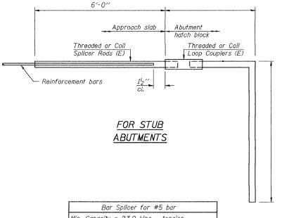
Min. Capacity = 23.0 kips - tension Min. Pull-out Strength = 12.3 kips - tension No. Required =
