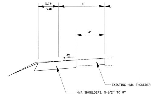
NOTE: FOR SHOULDER BUILD 5.5" AT STATION 663+00 AND 667+50 TO  $8^{\prime\prime}$  AT STATION 665+87 AND 670+59
