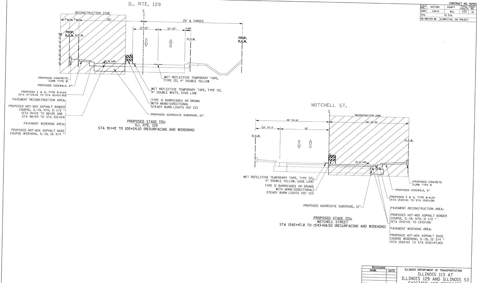
EXISTING AND PROPOSED TYPICAL SECTION STAGE IIIC
