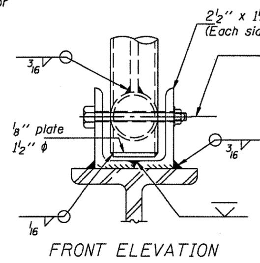
**The existing locking pin hole to be reamed for proper alignment and a new oversized stainless steel pin to be installed.**
