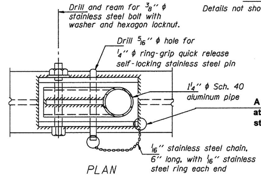
**A new stainless steel chain shall be attached to the angle with a 1/16" stainless steel ring.**
