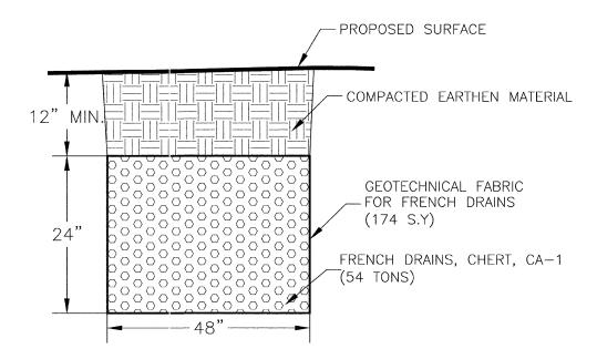
FRENCH DRAIN DETAIL DETAIL D-43 - NOT TO SCALE
