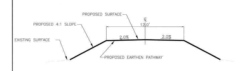
TYPICAL SPUR ROAD SECTION DETAIL DETAIL C-43 - NOT TO SCALE
