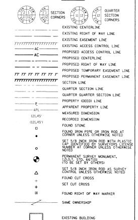
■ STAKING OF PROPOSED RIGHT OF WAY AND PERMANENT EASEMENT CORNERS. SET 5/8 INCH METAL ROD WITH DIVISION OF HIGHWAY SURVEY ALUMINUM CAP TO MONUMENT THE POSITION SHOWN, IDENTIFIED BY INSCRIPTION DATA AND SURVEYORS LICENSE NUMBER. (PROPOSED RIGHT OF WAY CORNERS SET IN CULTIVATED AREAS SHALL BE A MINIMUM OF 20 INCHES BELOW THE GROUND SURFACE).
