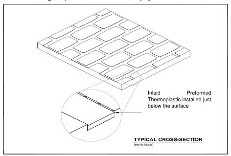
1.3. When applied in accordance with the manufacturer's application guidelines by an applicator certified by the manufacturer, the inlaid preformed thermoplastic will wear at a similar rate as the surrounding asphalt pavement. Therefore, the life of the inlaid preformed thermoplastic is dependent upon using a long lasting, durable and stable asphalt pavement to prevent premature wear.
