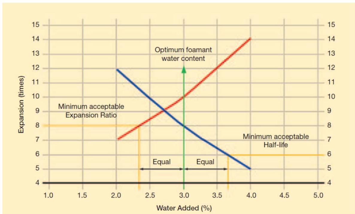
Repeat Steps 1 through 9 for two other bitumen temperatures normally 340 °F (170 °C) and 360 °F (180 °C). The temperature and optimum water addition that produces the best foam is then used in the mix design procedure described below.
