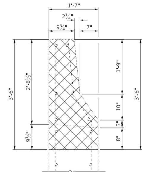
**CROSS SECTION THRU WING WALL**
