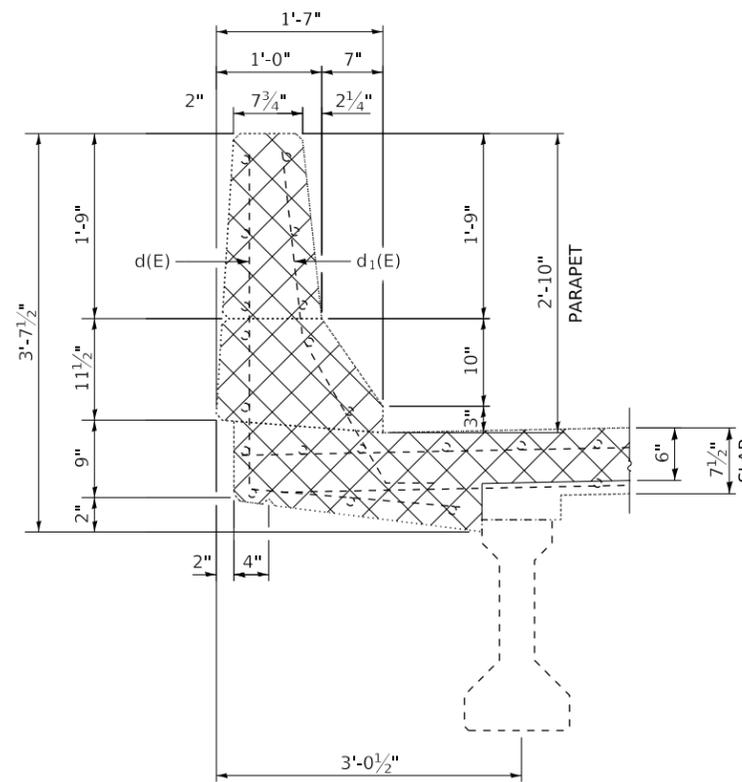
**CROSS SECTION THRU PARAPET**
