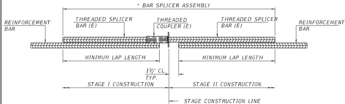
**STANDARD BAR SPLICER ASSEMBLY PLAN**
