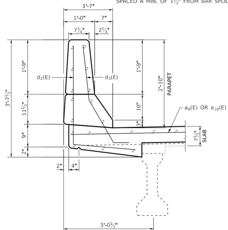
**CROSS SECTION THRU PARAPET**
