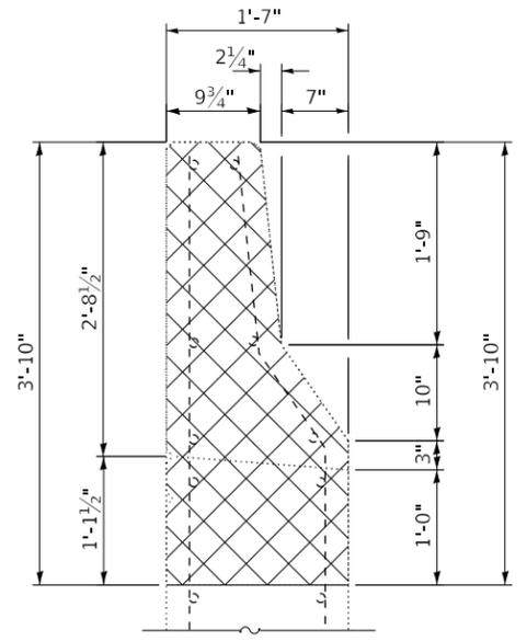
**CROSS SECTION THRU WING WALL**
