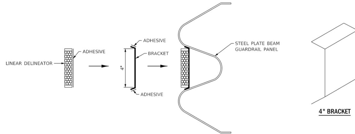
**LINEATOR DELINEATOR APPLICATION TO STANDARD GALVANIZED GUARDRAIL**
