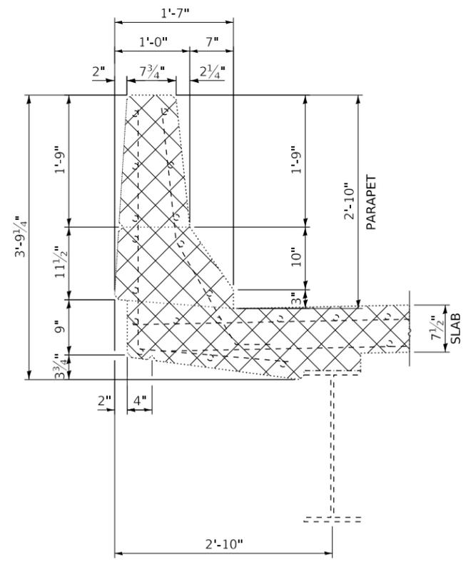
**CROSS SECTION THRU PARAPET**
