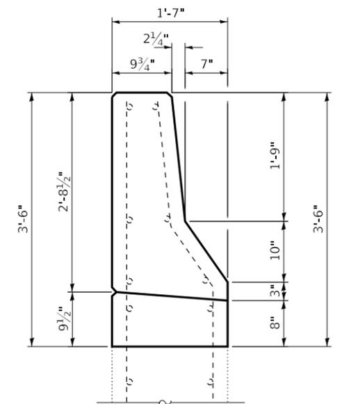
**CROSS SECTION THRU WING WALL**
