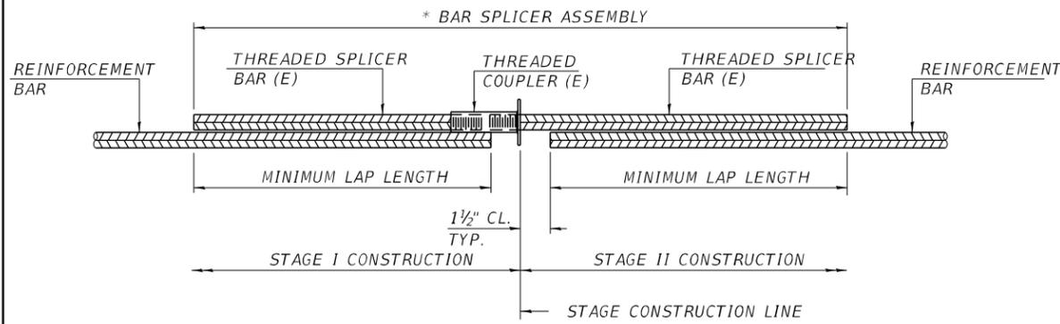
**STANDARD BAR SPLICER ASSEMBLY PLAN**
