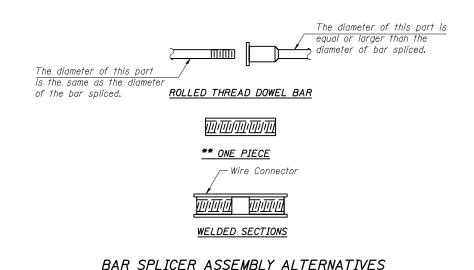
\*\*Heavy Hex Nuts conforming to ASTM A 563, Grade C, D or DH may be used.
