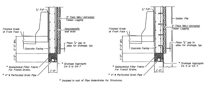
\* 4" | Perforated Drain Pipe
