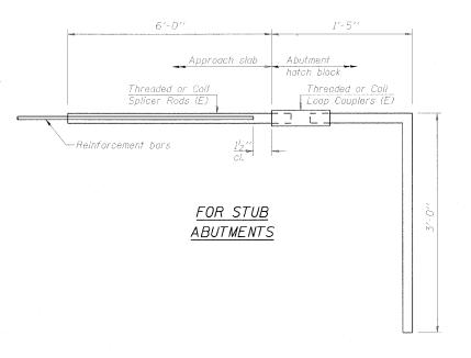
Bar Splicer for #5 bar fin. Capacity = 23.0 kips - tension n. Pull-out Strength = 12.3 kips - tension Required = 94
