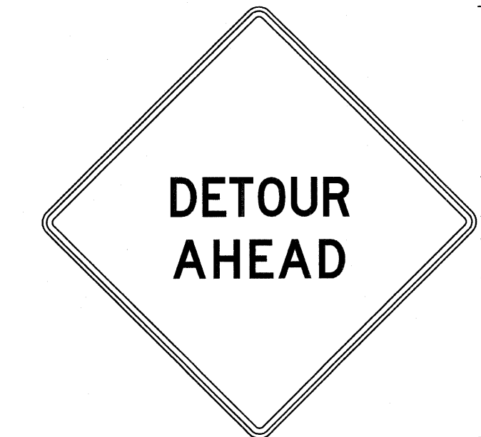
W20-2 MIN; 48.0" across sides 2.3" Radius, 0.9" Border, 0.6" Indent, Black on Orange; [DETOUR] D 60% spacing; [AHEAD] D 102% spacing;
