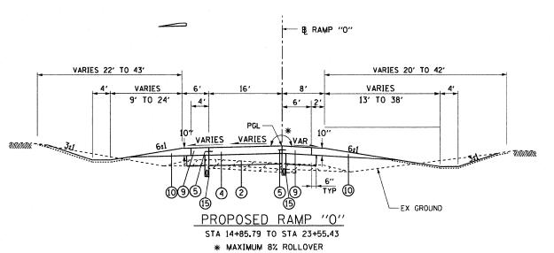
FULL SUPERELEVATION - STA 14+60.05 TO STA 17+89.35 (8.0% RT) STA 21+43.77 TO STA 22+72.20 (6.0% LT)
