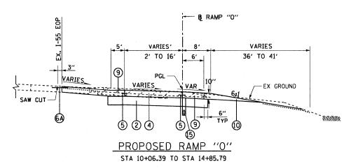
SUPERELEVATION TRANSITION - STA 12+92.30 TO STA 14+60.05 (1.5% LT TO 8.0% RT)
