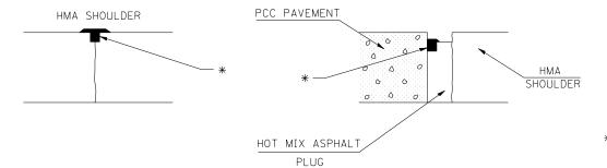
\* HOT ASPHALT CRACK ROUTING 3/4 " x 3/4" x LENGTH OF CRACK, AS NEEDED. FIBER ASPHALT LEFT FLUSH WITH PAVEMENT.
