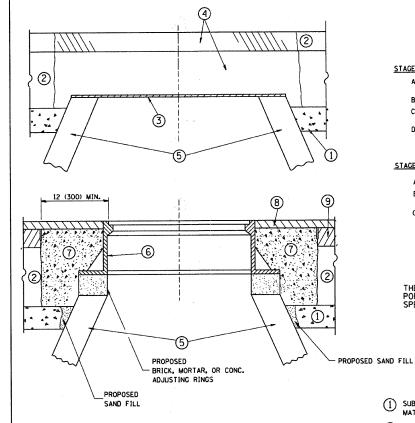
EXISTING BROKEN FRAMES AND LIDS SHALL BE REMOVED AND DISPOSED OF BY THE CONTRACTOR AND SHALL BE REPLACED AS DIRECTED BY THE ENGINEER. REPLACEMENT FRAMES AND LIDS WILL BE PAID FOR IN ACCORDANCE WITH ARTICLE 109,04 OF THE STANDARD SPECIFICATIONS UNLESS A SEPARATE PAY ITEM HAS BEEN PROVIDED.
